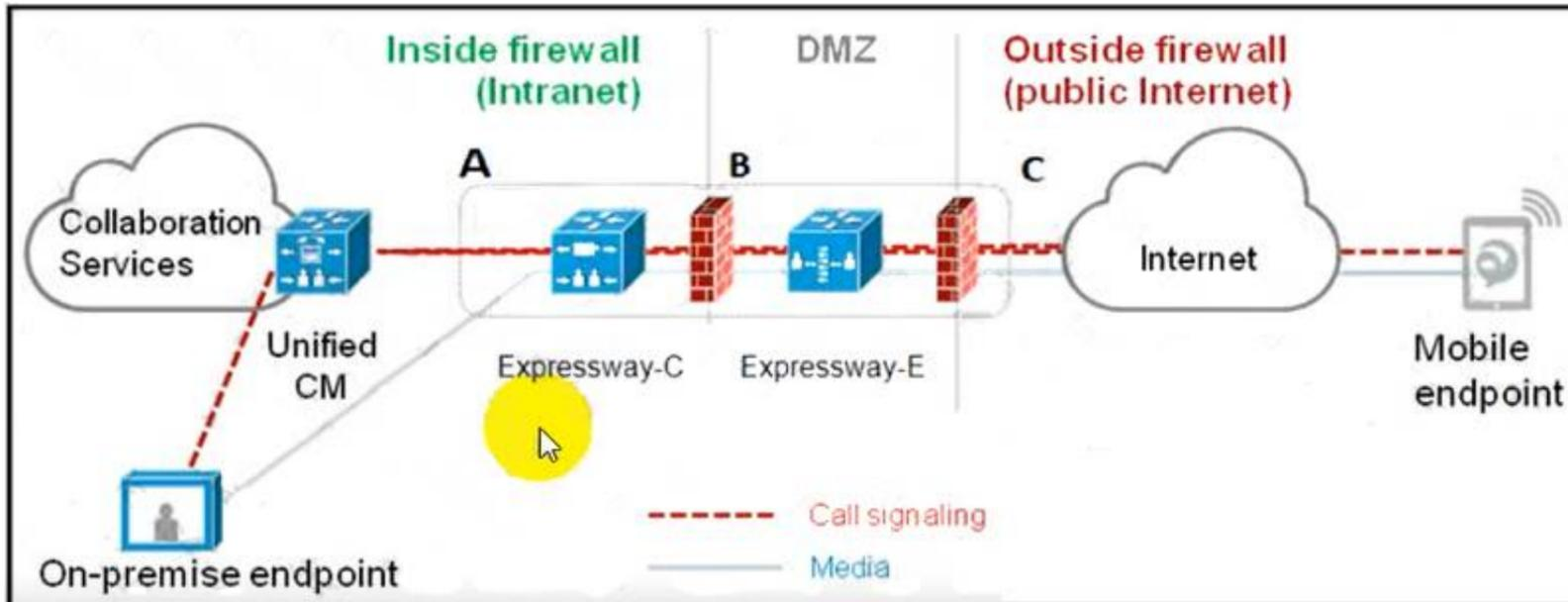
When making a call to a Mobile and Remote Access client, what are the combinations of protocol on each of the different sections A-B-C?
