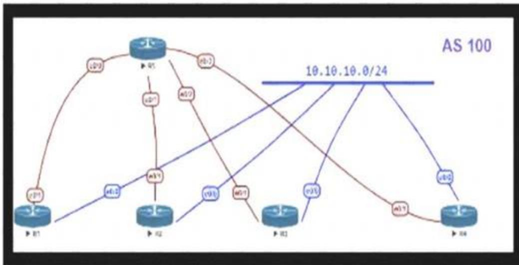
OSPF is running as the IGP to provide reachability to all AS100 networks R3 and R4 are the current ABRs at the boundary of OSPF Area0 and Area1 Now BGP must be deployed within AS 100 because it will be receiving Internet routes from its eBGP peers (the service provider) connected to R1 and R2 What is an optimal solution for this deployment to configure BGP relationships and redistribute BGP learned routes into OSPF?
