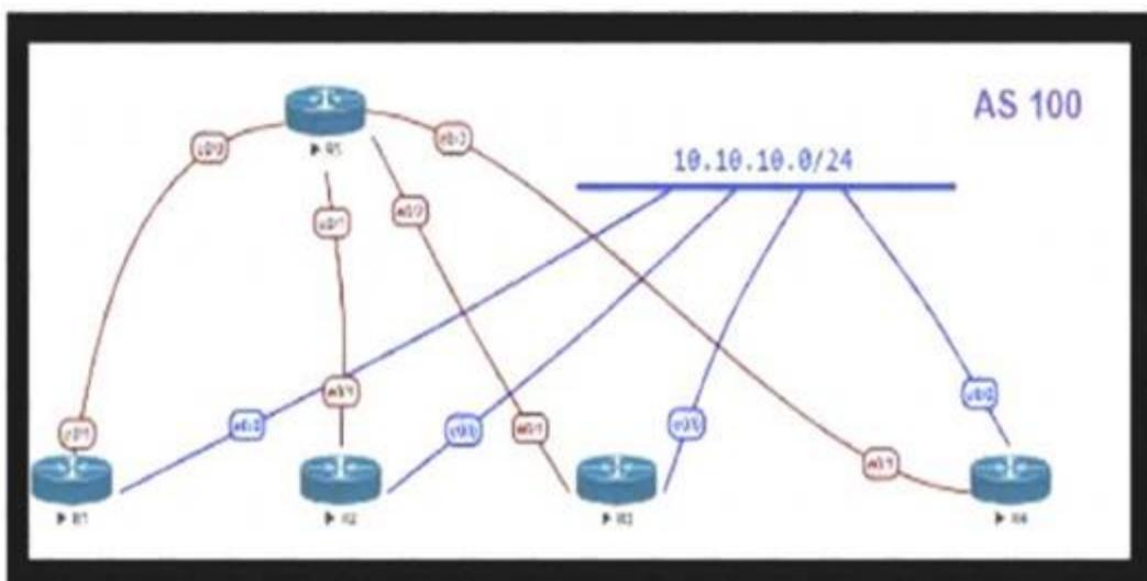
OSPF is running as the IGP to provide reachability to all AS100 networks. R3 and R4 are the current ABRs at the boundary of OSPF Area 0 and Area 5. Now BGP must be deployed within AS 100 because it will be receiving Internet routes from its eBGP peers (the service provider) connected to R1 and R2. What is an optimal solution for this deployment to configure BGP relationships and redistribute BGP learned routes into OSPF?
