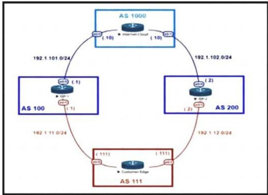
An engineer is designing the traffic flow for AS 111. Traffic from AS 111 should be preferred via AS 100 for all external routes. A method must be used that only affects AS 111. Which BGP attributes are best suited to control outbound traffic?
