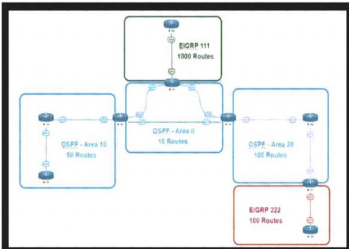
This network is running OSPF and EIGRP as the routing protocols. Mutual redistribution of the routing protocols has been configured on the appropriate ASBRs. The OSPF network must be designed so that flapping routes in EIGRP domains do not affect the SPF runs within OSPF. The design solution must not affect the way EIGRP routes are propagated into the EIGRP domains. Which technique accomplishes the requirement?
