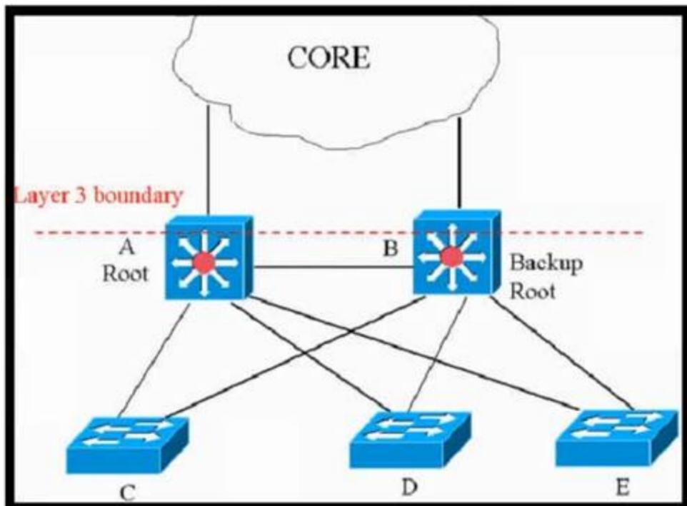
This network is running legacy STP 802.1 d. Assuming "hello\_timer" is fixed to 2 seconds, which parameters can be modified to speed up convergence times after single link/node failure?
