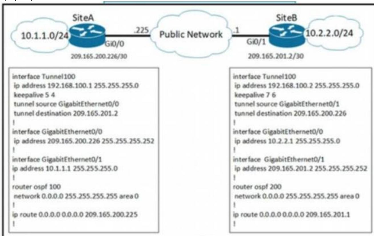
A network engineer configures a new GRE tunnel and enters the show run command. What does the output verify?
