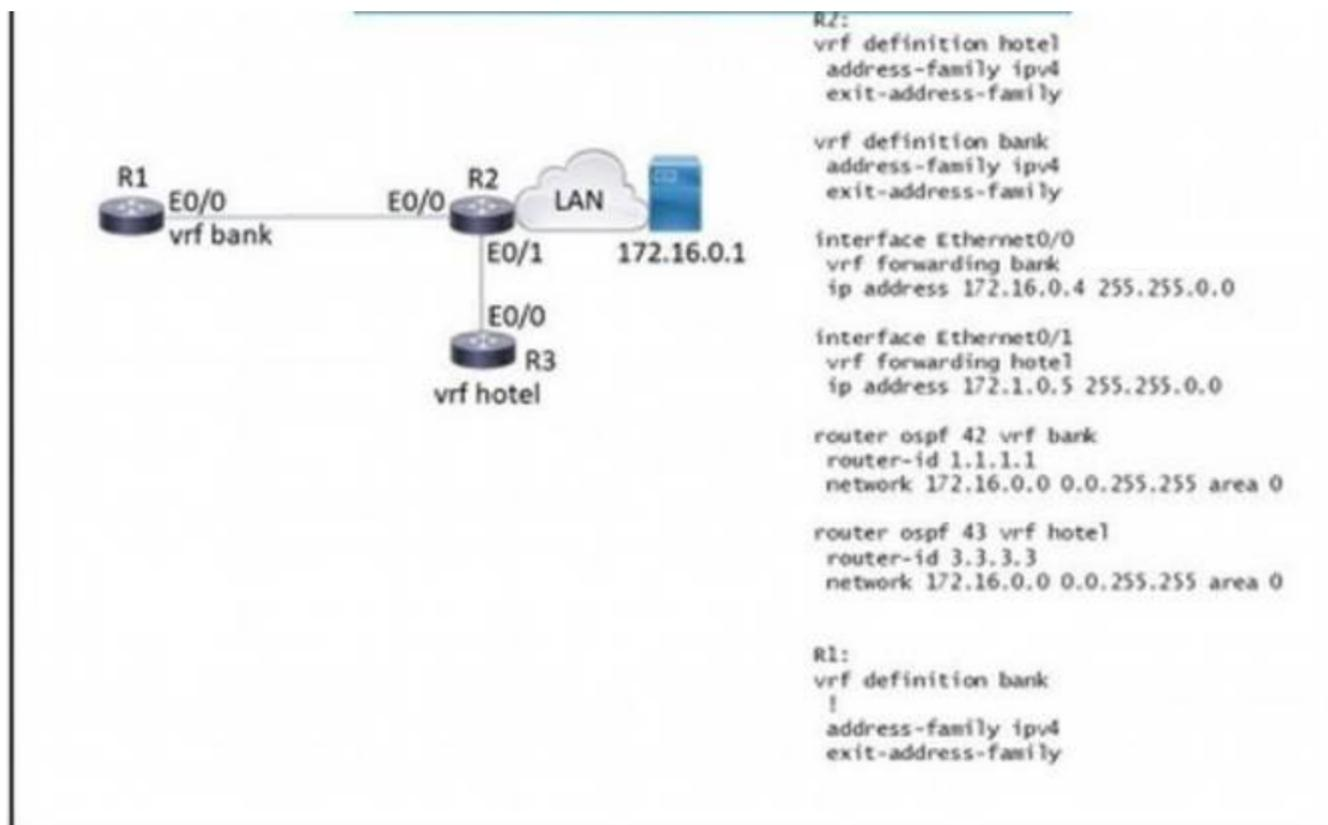
Refer to the exhibit. Which configuration must be applied to R1 to enable R1 to reach the server at 172.16.0.1?
