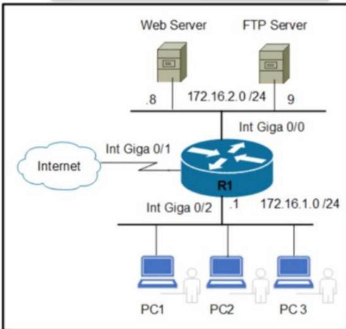
Refer to the exhibit. An engineer must allow the FTP traffic from users on 172.16.1.0 /24 to 172.16.2.0 /24 and block all other traffic. Which configuration must be applied?
