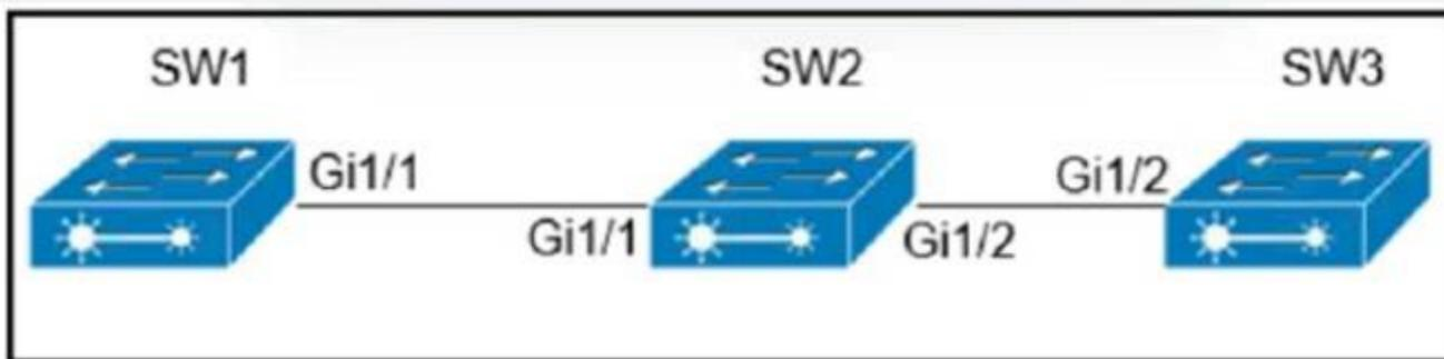
Company policy restricts VLAN 10 to be allowed only on SW1 and SW2. All other VLANs can be on all three switches. An administrator has noticed that VLAN 10 has propagated to SW3. Which configuration corrects the issue?
