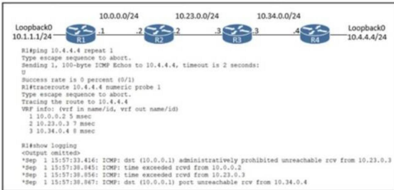
Refer to the exhibit. What is the cause of the communication failure between R1 and R4?
