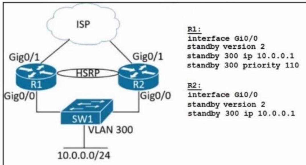
Refer to the exhibit. An engineer must implement HSRP between two WAN routers. In the event R1 fails and then regains operational status, it must allow 100 seconds for the routing protocol to converge before preemption takes effect. Which configuration is required?
