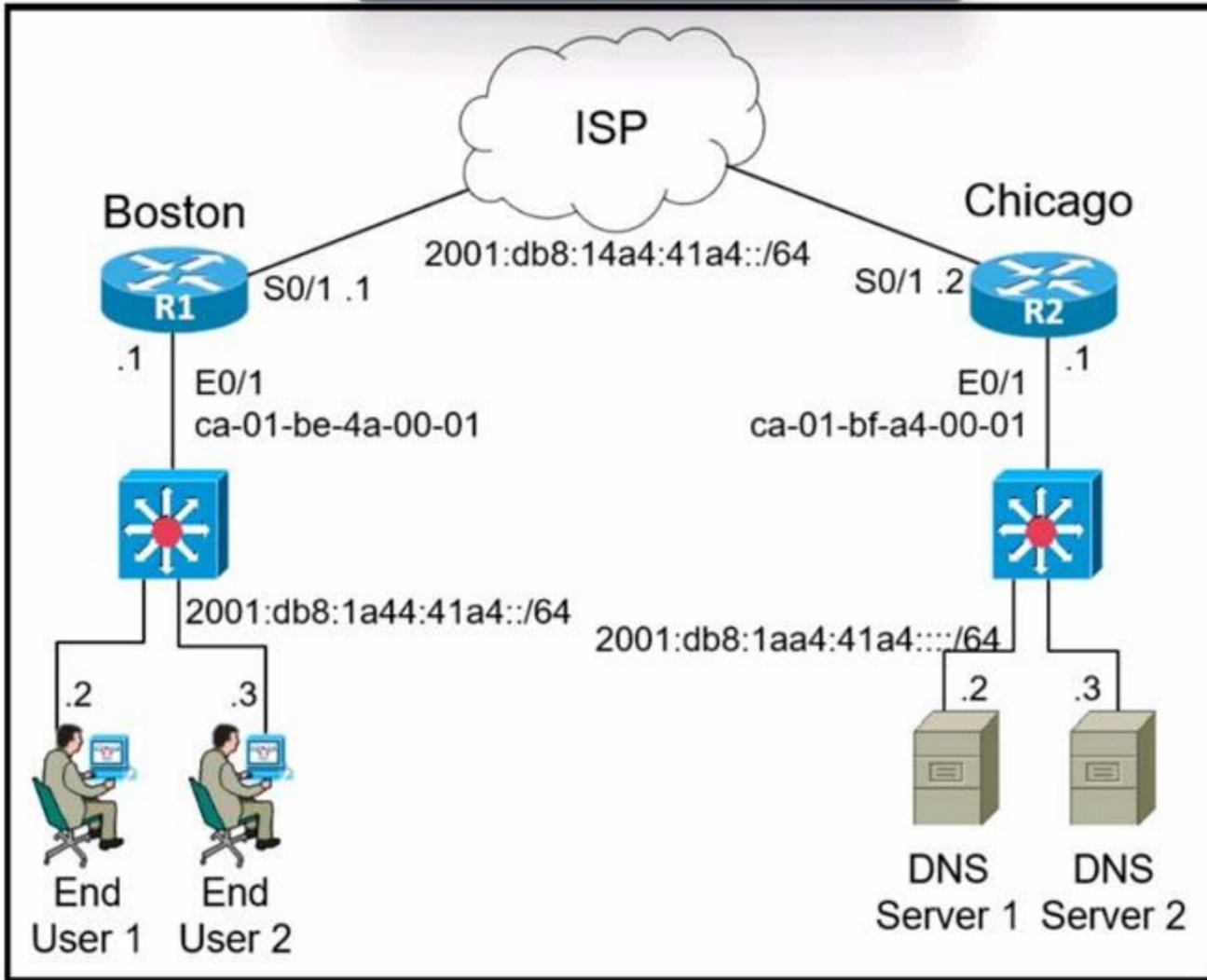
Refer to the exhibit. The IPv6 address for the LAN segment on router R1 must be configured using the EUI-64 format. When configured which ipv6 address is produced by the router?
